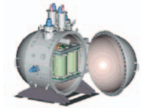
Fig. 4: A Schematic design of SMES [24]
